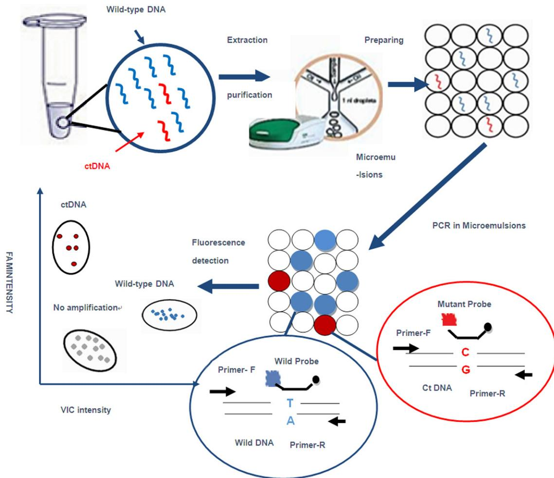
**Figure 2.** Schematic illustration of ctDNA analysis by droplet digital-PCR [20].
